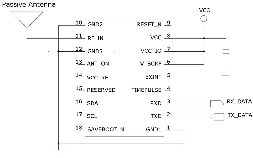
2. Example 2 for GPS/GLONASS Passive Antenna and External LNA
