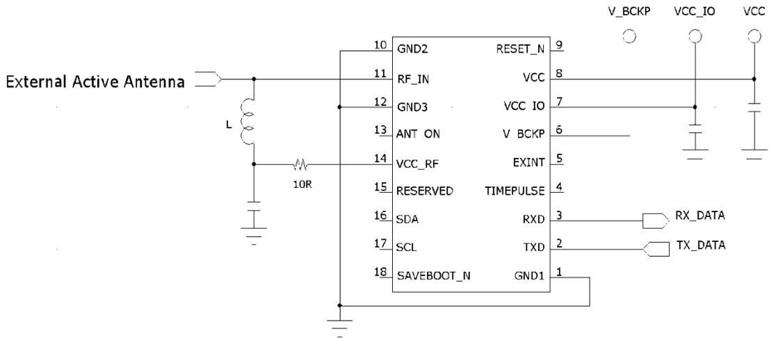
4. Example 4 for GPS/GLONASS external Active Antenna using Supply from External Supply
